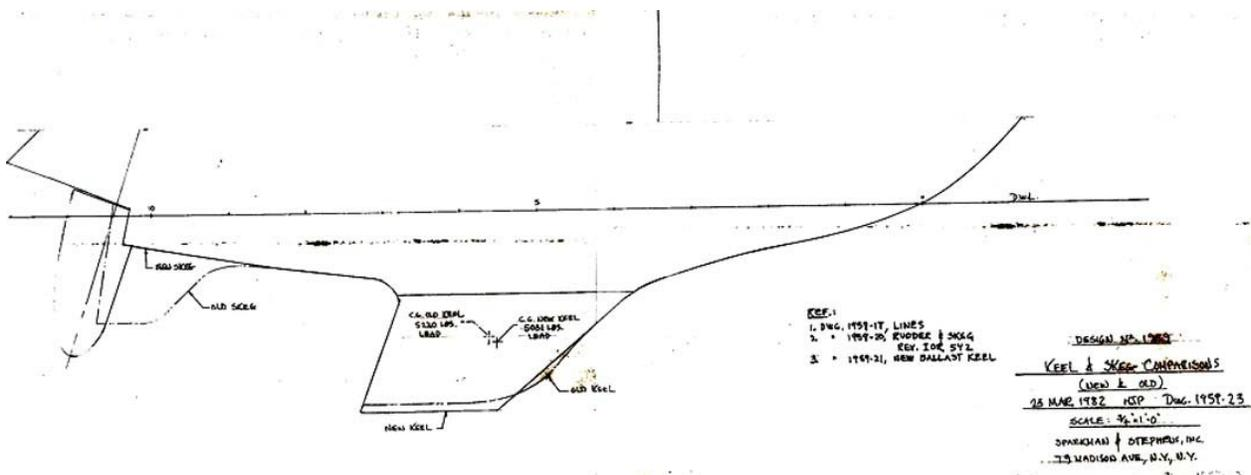
*Drawings showing the differences between Mk I and Mk II keel profiles*
