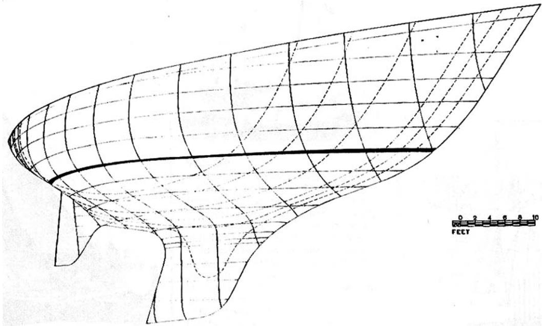
*Mk ! keel and sloop isometric drawing*
