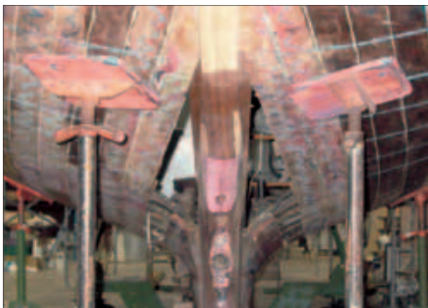
Horn Timber renewed
