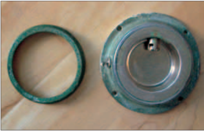
Old corroded Perko light fittings
