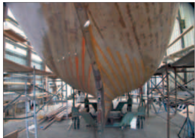
Planked up and caulked
